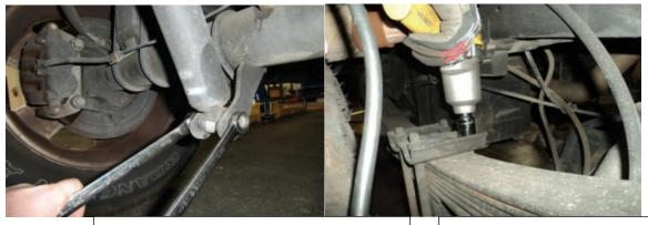
Remove the lower shock mount hardware.
