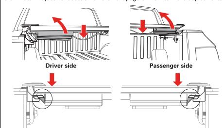
**13** Retighten the cover retainer clamps once the desired fitment is reached. You are ready to drive with your cover in the closed position.
