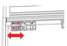
With the latch cover removed, loosen the screws and move the latch bracket to adjust. Retighten the screws. Slide the latch housing back on.
