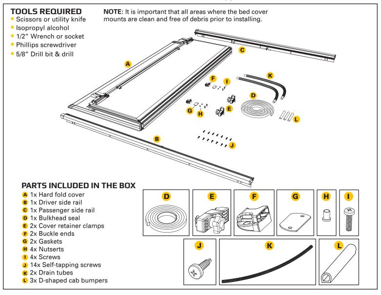
**Installing Seal**: Bulkhead seal (D) is included with the cover (A), clean the top of the bulkhead with soap and water to remove dirt and debris. Clean the area with isopropyl alcohol to remove wax or grease and to evaporate any remaining water. Allow the surface to dry. Peel the
