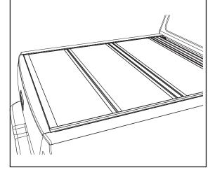
**OPENING COVER:** Lower the tailgate and pull the cable on either side. While pulling on the cable lift the panel up and towards the cab.
