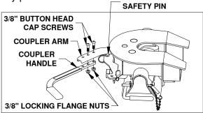
Figure E1: View looking down at side of coupler.
