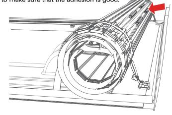
Install one end cap (C) on the rearward portion **ONLY** of the new passenger side cover rail (A), as shown. Tighten the set screw with the provided Allen wrench. Do this also on the new driver side cover rail (B).
