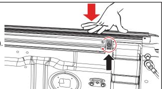
With both rails (A & B) clamped in place, rest the rolled cover (E) onto the rails at the tailgate, roll the cover toward the cab, and remove and discard all packaging materials.
