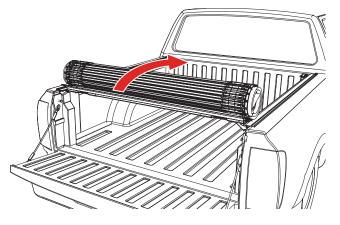
Fold the front panel back and insert the two mounting bolts (L) into the slotted bracket. Do this for both sides. The bolts will align with the slotted bracket of the cover rail. Fold the panel back down.
