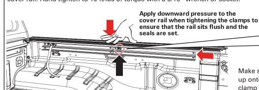
Make sure that the clamps are inserted as far up onto the cover rail as possible and that the clamp feeth fit squarely and fully engage the ribs of the cover rail.
