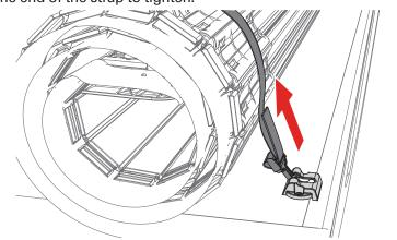
**CLOSING COVER:** Roll the cover (E) toward the tailgate and rotate the tail rail downwards towards the rotating locking levers.
