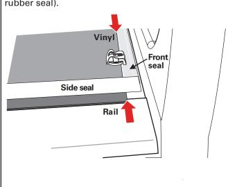
Verify that a gap of approximately 1/8" (3.2mm) remains on both sides of the cover (E) between the edge of the cover rail and the rolling cover. This spacing is necessary to ensure that the locking rail secures to cover. Align the cover side to side at the front and/or the back if the side gaps are not even. Firmly hand tighten the knobs (I) after the cover has been aligned.
