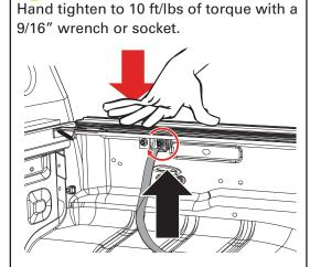
FOR TRUCKS WITH CARGO RAILS: Insert the provided strap clamp (F) above the cargo rail at the rear. Slide the strap clamp as far forward as possible. Hand tighten to 10 ft/lbs of torque with a 9/16" wrench or socket.
