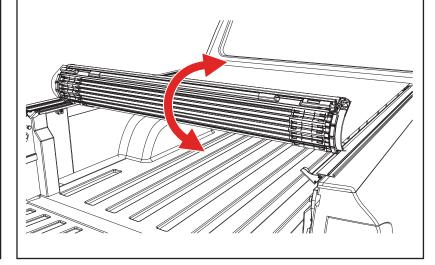
Align the front vinyl edge of the rolled cover (E) with the front edge of the side rails (not the rubber seal).
