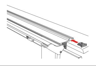
**ROLLED UP POSITION:** To drive with the cover (E) in the open position, use the strap clamps. Roll the cover forward, twist and insert the clips into the cover clasps. Ensure that BOTH strap clamps are fully inserted into the clasps. Pull on the end of the strap to tighten.
