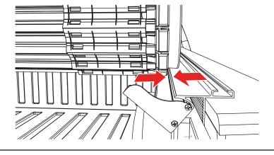
When correctly installed, the vinyl edges of the cover (E) will align squarely with the side rails in all four corners. The latch assembly will align with the side rail locking levers at the tailgate on both sides.
