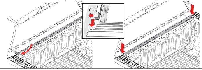
Position the new passenger side cover rail (A) on the truck rail with the slotted bracket pushed all the way toward the front/cab and the bulkhead.
