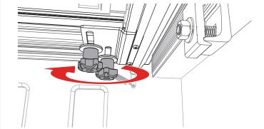
When the cover (E) is in the open position, the other end of the strap clamp assembly (F) inserts into the cover clasp and turns to lock. Pull up on the strap end to tighten. Always hook the straps on BOTH sides.
