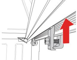
Place the second clamp (G) near the center of the cover rail. For 8' beds, two clamps will be evenly spaced in the center section of the cover rail. Hand tighten to 10 ft/lbs of torque with a 9/16" wrench or socket.
