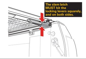
Check to see that the latches on both sides at the tailgate fully engage the cover rails (A & B).
