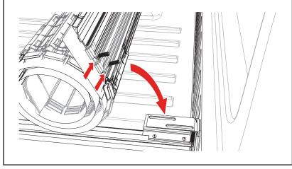
Install the mounting hardware from step 2 loosely underneath the slotted bracket on the passenger cover rail (A). Start with the rubber washer (K), then the large flat washer (J), then hand tighten the lock knobs (I). Repeat on the driver's side. Leave the knobs loose for now.
