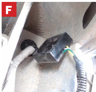
F ROUTE WIRE HARNESS THROUGH UP TO THE CONTROL BOX
