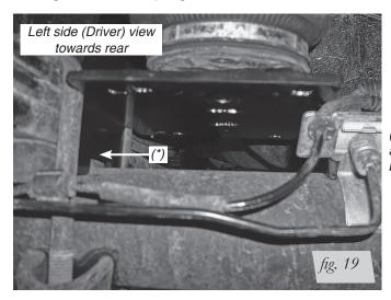
(\*) Push the bracket against the leaf spring in between the stock U-bolts.
