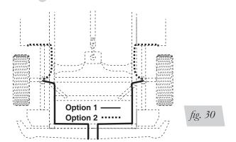
7. Cut off the air line, leaving approximately 12" of extra air line. A clean square cut will ensure against leaks. Insert the air line into the air fitting. This is a push-to-connect fitting. Simply push the air line into the 90° swivel fitting until it bottoms out (9/16" of air line should be in the fitting).
