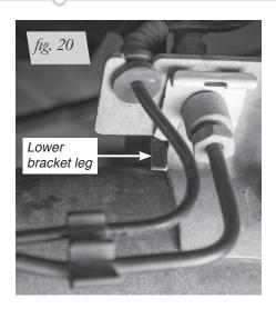
7. Insert the long carriage bolts (T) into the bottom bracket.
