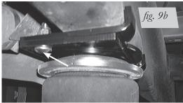
Right hand assembly (passenger side) attached with carriage bolts (R), flat washers (M) and nylon lock nuts (U). Torque to 31 lb.-ft.
