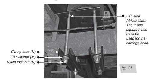
Install the lower clamp bars (N) over the carriage bolts installed previously and cap with flat washers (M) and nylon lock nuts (U) (Fig. 11). Torque the lower nuts evenly to 10 lb.-ft.
