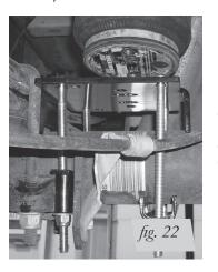
Right side (passenger) view towards front of finished installation torqued to 10 lb.-ft.
