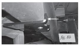
RH (passenger) side. Push bracket against frame and torque to 38 lb.-ft.
