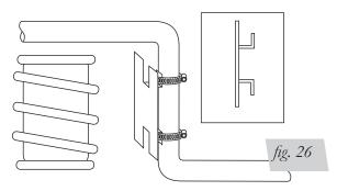
4. Bend the heat shield to form it around the tail pipe. Be sure to maintain a "dead air" space of 1/2" to 1" between the tail pipe and the heat shield (Fig. 27).
