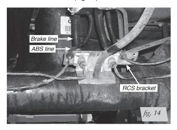
2. Remove the right ABS line out of the bracket by pulling it straight up (Fig. 15).
