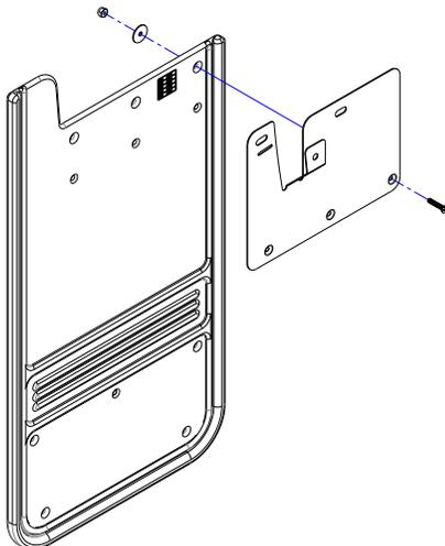
5. Now secure the flap with a flat washer and a tek screw on hole #2 through the wheel tub.
