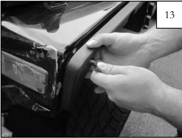
As you line up the inner piece, feed the wire harness through the hole in the front of the bracket.
