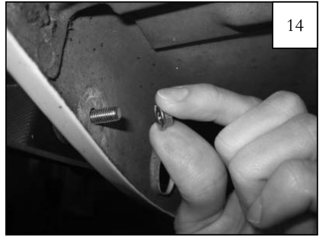
Attach flange nuts (NU1-0010) to the threads on the M5-.8 machine screws and hand tighten.
