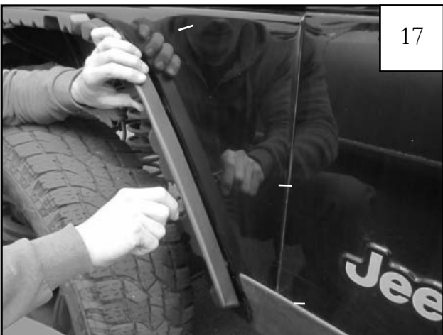
While holding the inner piece in place, use a #2 Phillips bit to tighten the M5-.8 machine screws (SW1-0053) into the factory mounted nuts (NU1-0010).
