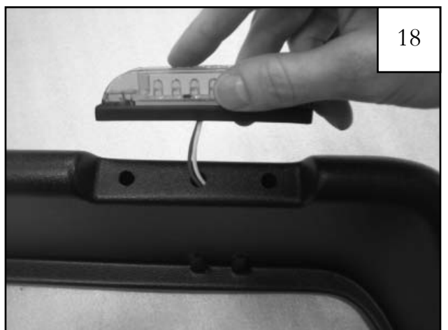
Position the supplied side marker light (LT1-0003) onto the outer flare piece, threading the wires through the center predrilled hole.
