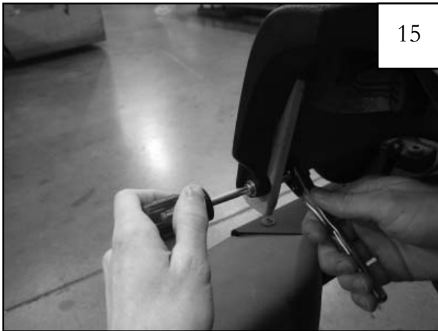
Fully tighten flange nuts using a 5/16" socket and wrench and use a #2 Phillips bit for the M5-.8 machine screws.
