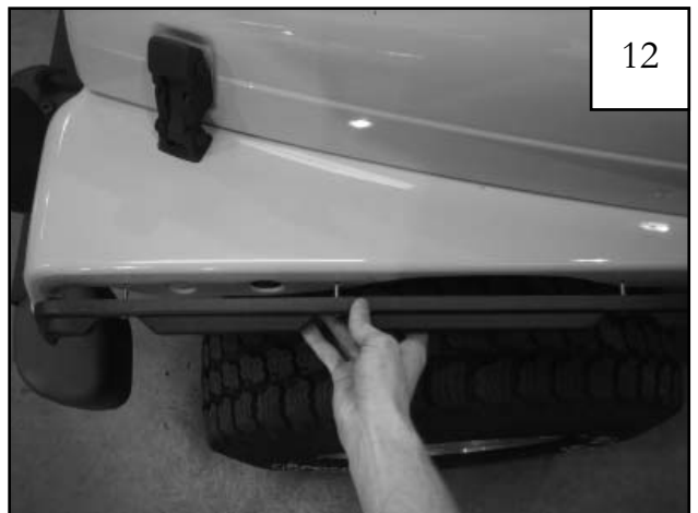
12 Secure inner piece D1 (and P1 for passenger side installation) to the sheet metal using the following Line up the M5-.8 machine screws (SW1-0053) with the factory hole locations and push them into place.
