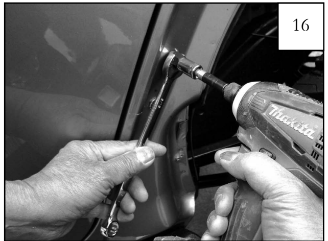
Using a wrench to hold rivnut tool in place, install rivnut in place on fender using an 11/16" socket. The rivnut will expand to secure itself in place. NOTE: Use of impact driver recommended for rivnut installation.
