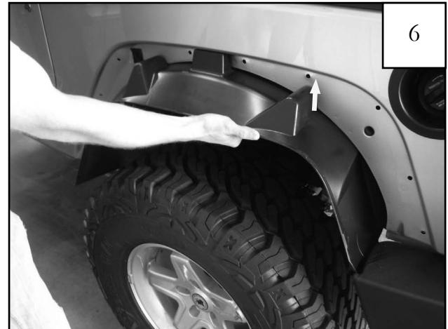
Hold the splash shield in place using supplied 1/4" Panel Retainers through factory holes halfway. Do not fully install Retainers, leave them half out. They are only used to hold splash shield in place for marking.
