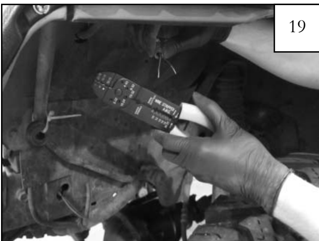
Use wire strippers to strip away approximately 3/8" of wire covering from the factory installed side marker lamp wires.
