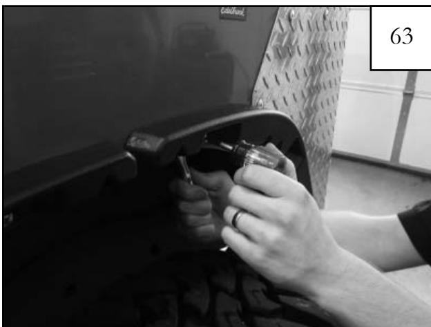
Step 4 Fully tighten Nuts (NU1-0010) using a 5/16" socket wrench and a # 2 Phillips bit for the Screws (SW1-0053).
