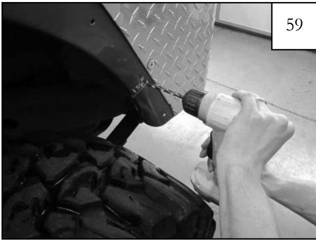
Using a 1/4" drill bit, drill marked hole.
