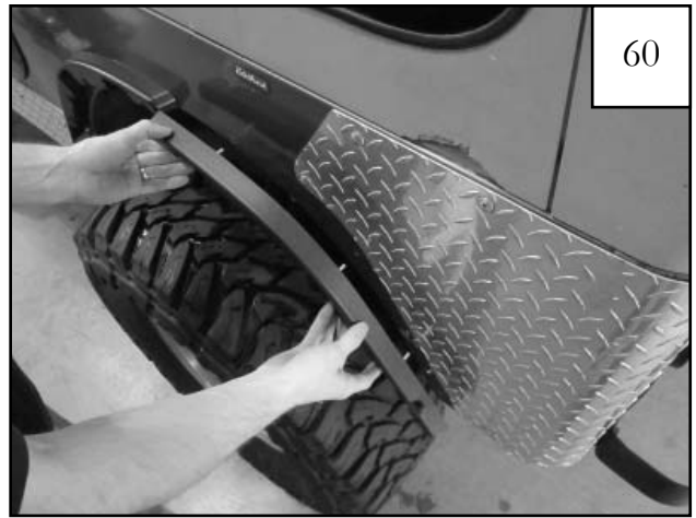
Secure inner piece D4 (P4 for passenger side) to the sheet metal using the following 4 STEPS : Step 1 Line the Screws (SW1-0053) and Washers (WA1-0003) with the factory hole locations and drilled hole.
