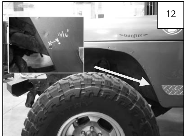
Locate the second factory hole from bottom of fender. Use a grease pencil to mark a hole for drilling 11/16" from center of factory hole, perpendicular with wheel well opening.
