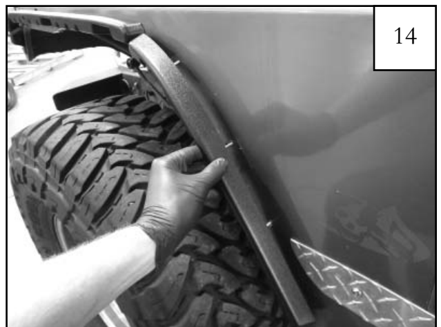
Secure inner piece D2 (and P2 for passenger side installation) to the sheet metal using the following 2 Steps: Step 1 Line up the three Screws (SW1-0053) with the upper factory hole and two drilled locations.
