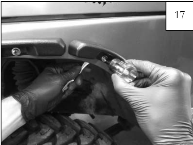
Step 3 Fully tighten Nuts (NU1-0010) using a 5/16" socket wrench and a # 2 Phillips bit for the Screws (SW1-0053).
