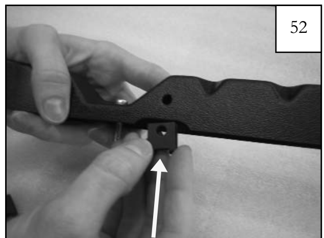
Install a Clip (CL1-0022) at each Clip location on the inner pieces, centering them on the predrilled holes. (6 locations)
