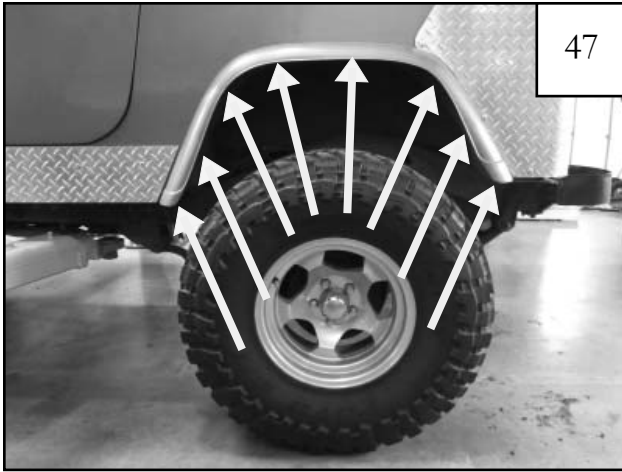
Remove the factory installed fender flare screws with a 5/16" socket wrench. (8 locations)
