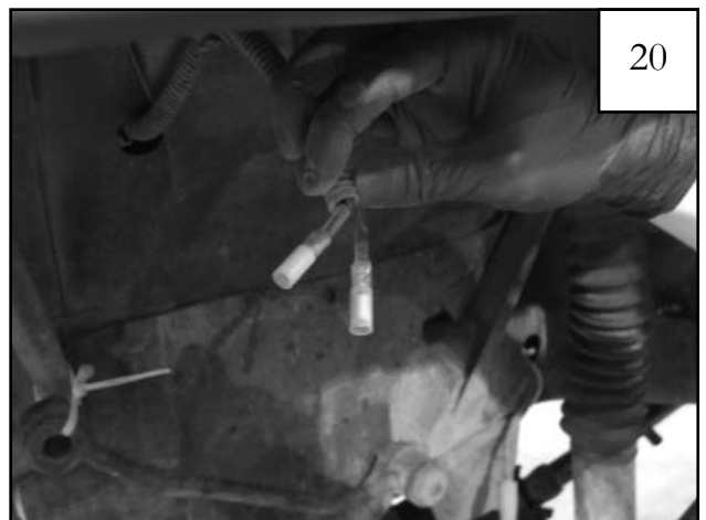
Install a Connector (EC1-0007) to the end of each factory side marker light wire and secure by pressing firmly with a wire crimp.
