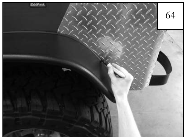
OPTIONAL: If aftermarket corner panels or rocker pieces are installed, you may need to trim them for a proper fit. If so, place main flare over inner pieces and use a grease pencil to mark them for trimming. Then remove flare and trim as needed.
