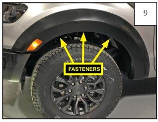
Reconnect the turn signal wiring connector and set the flare in place. Hold flare to vehicle and install (3) 1/4" panel retainers (RV1-P008) into the wheel well holes indicated. Press firmly on the flare while installing fasteners.
