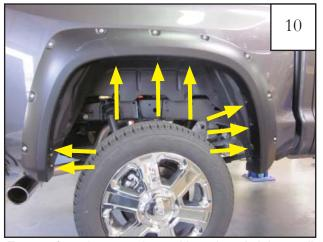
Ensure flare is properly positioned and tighten all screws. (See steps 6-8). Installation Complete
