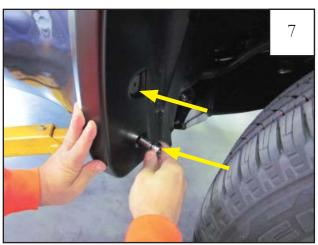
Start two supplied 20mm Hex Screws (SW1-0036) through the rearward most holes of flare and into the factory hole in fender.
