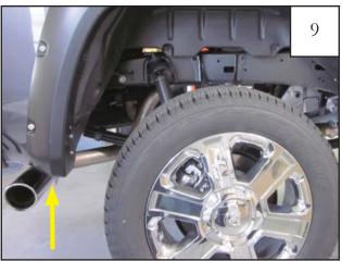
Install supplied Push Retainer (RV1-P009) into factory hole on underside of flare.
