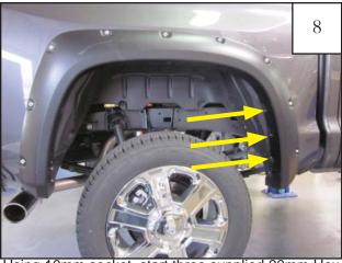
Using 10mm socket, start three supplied 20mm Hex Screws (SW1-0036)through the forward most holes of flare and into factory holes in fender.
