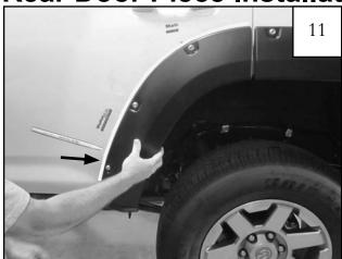
NOTE: Clean factory door piece installation surfaces with a soft cloth and mixture of 50/50 water and isopropyl alcohol.
