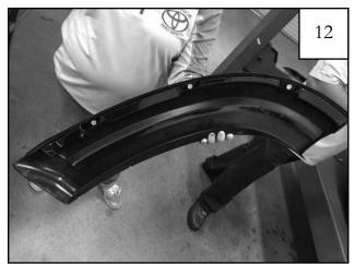
Remove tape liner from all tape on back of door piece.
