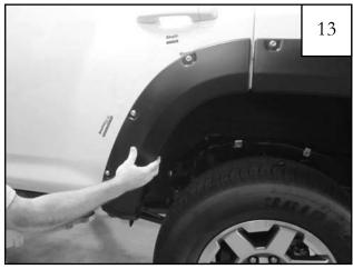
NOTE: You cannot remove the door piece once it has stuck to the vehicle.
