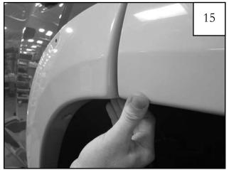
Align door piece with rear flare before drilling and installing screws.
