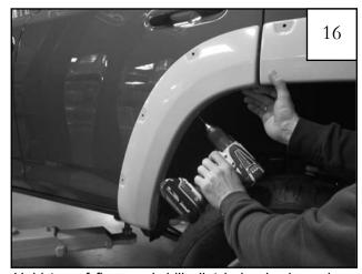
Hold top of flare and drill pilot holes in door piece with 1/8" bit.
