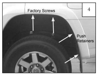
Remove two factory screws and two factory push retainers from the Rear Main Flare ONLY. Retain screws for reinstallation.
