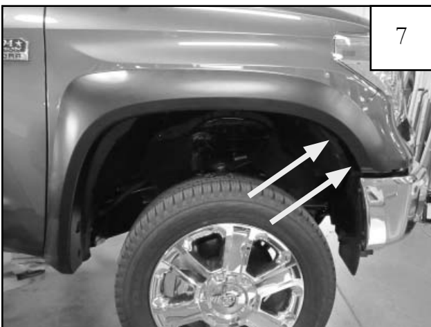
7 Start two supplied 20mm Hex Screws through front most holes in flare and into factory hole locations.
