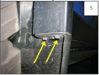
Remove two bolts connecting factory flare to rocker as shown (one plastic fastener removed in Step 4 is located here as well).
