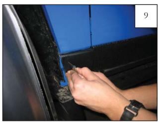
Trim an additional 3/4" from rocker, so that end of rocker is within confines of sheet metal. *NOTE: The Flare will cover this area to 1/4" from the door seam.*
