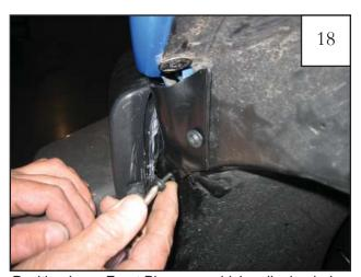
Position Inner Front Piece on vehicle, aligning holes in part with holes in Clips installed in previous Step. Install supplied Screws (SW1-0056).
