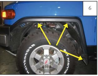
Remove three plastic fasteners using a flat head screw driver or pry tool.
