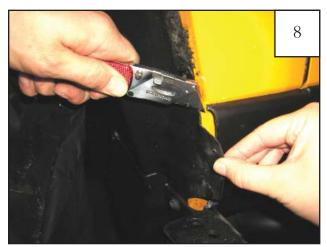
Using a utility knife, cut splash guard flush with edge of sheet metal also.
