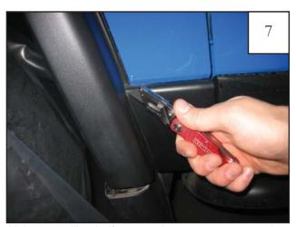
Using a utility knife, cut along seam connecting factory flare to rocker. Cut down to mud flap area.
