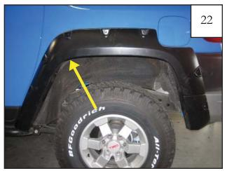
Install one supplied Fastener (RV1-P003) in top forward hole. Check that Edge Trim (GP1-0001) is seated correctly, then tighten all Screws.
