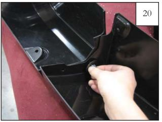
Slide a supplied Washer (WA1-0017) onto backside of Screw (SW1-0005), and thread a supplied Nuts (NU1-0001) onto Screw. Using a 10mm socket and 7/16" wrench, tighten Screws.
