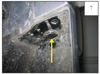
Remove one plastic fastener from mud guard.
