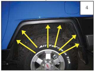
Using a 10mm socket, remove six bolts.
