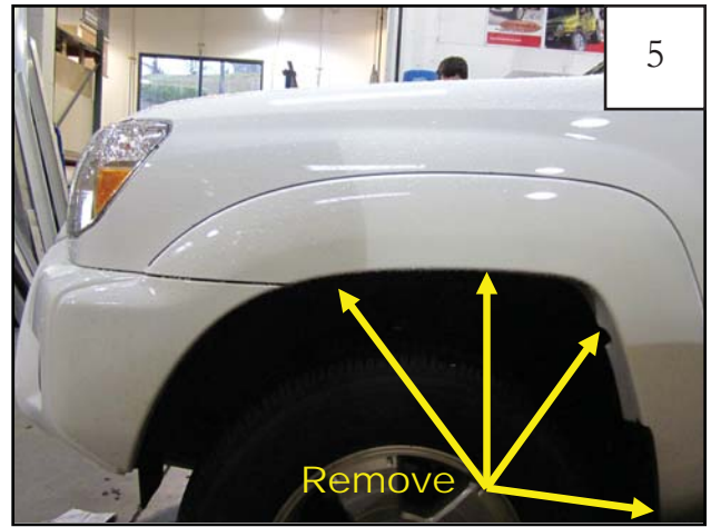
Remove four factory screws from the fender lip. Save screws for reinstallation. Remove flare by pulling part away from side of vehicle.
