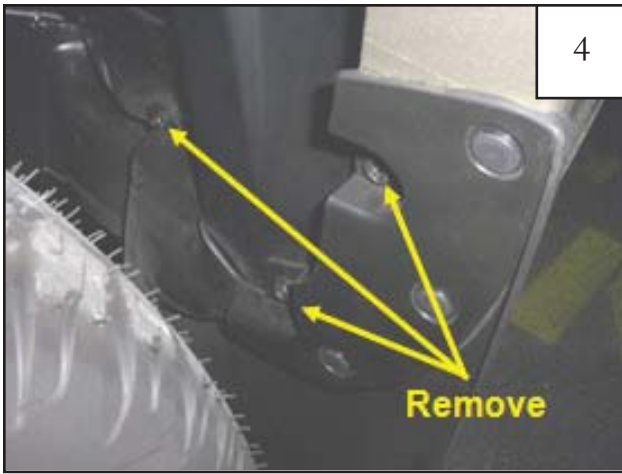
Remove three factory screws from the mud flap. Save screws for reinstallation.
