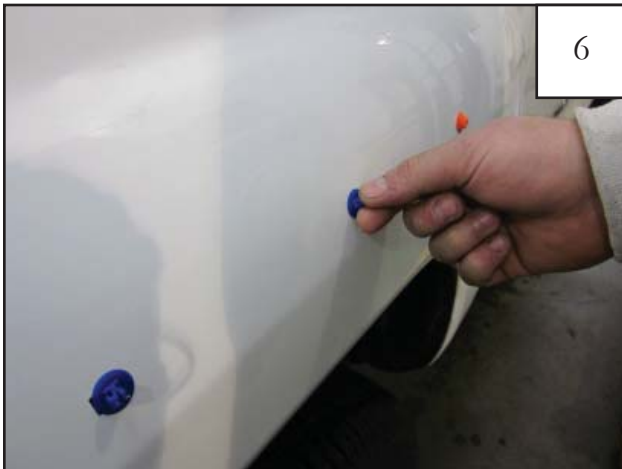
Using a clockwise twisting motion, remove eight factory plastic clips from fender. See step 8.
