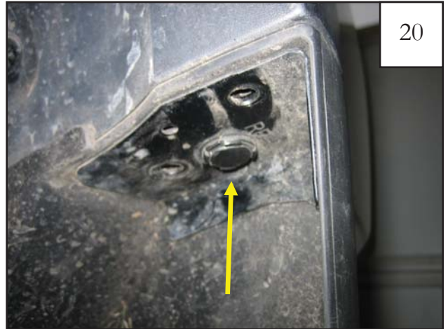
Remove one plastic fastener from mud guard.
