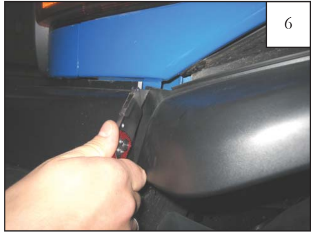
Cut front of factory flare along bumper, taking care not to cut bumper.
