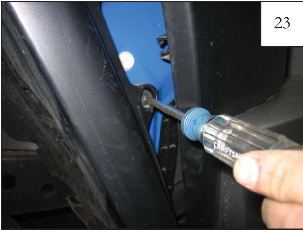
Remove bolt located behind rear plastic panel. Note: If the socket does not fit in the enclosed space, a phillips screwdriver will work.
