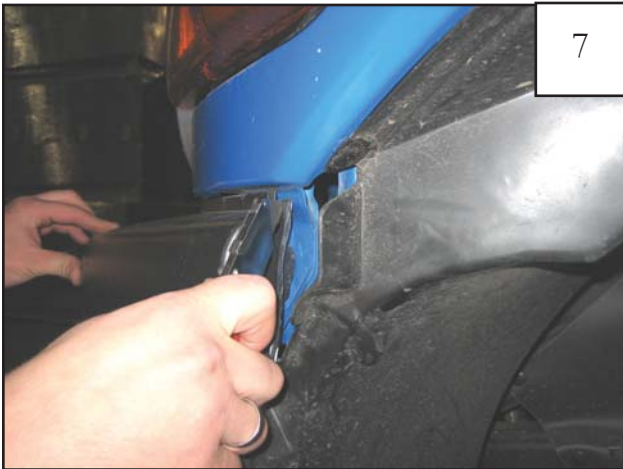
Trim remaining plastic flush with bumper.
