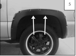
Hold rear flare in place on fender and start the top two Screws (SW1-0056), threading them through the flare, the Clips, and into the factory holes. *Do not tighten.*
