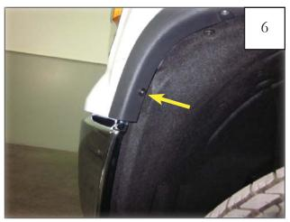
Remove fastener from front of factory wheel arch molding using a 9/32" or 7mm socket and wrench. Save for reinstallation.
