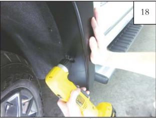
Install self-tapping screw (SW1-0066) into pilot hole drilled in step 16. Press flare towards vehicle while fully tightening. *Note: This step not needed for models with factory installed mudflaps.*
