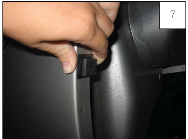
Slide a supplied clip over each black tab. Clips may need to be adjusted to align with holes in flare.
