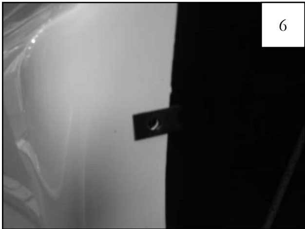
Install Clip (CL1-0011) over existing factory hole.
