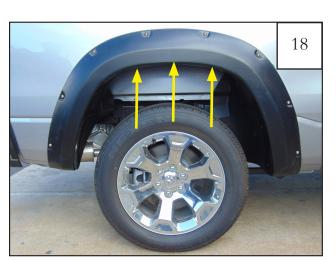
Hold flare in place and start Screw (SW1-0056) using a Phillips screwdriver in (3) locations as shown. *Do not tighten.* **Continue to Step 21.**
