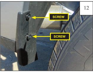
Remove and keep (2) factory installed screws, and remove mud flap from vehicle. These factory screws will be used to install the rear fender flare.
