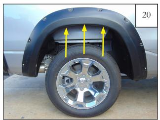
Hold flare in place and reinstall (3) factory screws removed in Step 19. *Do not tighten*.
