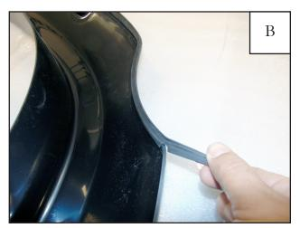
Cut a V in the edge trim at the fuel door cutout exit so the edge trim doesn't bulge when you wrap around the part.
