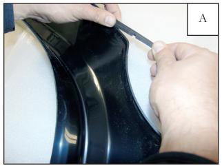
Start at the rear of the flare and work toward the front. Cut a V out of the edge trim's backside at the fuel door cutout's sharp curve so the edge trim doesn't bulge when you wrap around the part.
