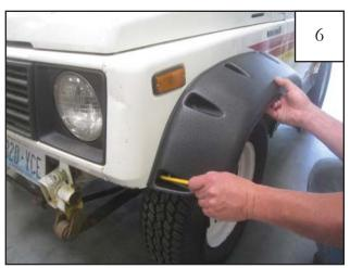
Hold front flare in position on fender and, using a grease pencil, mark each hole location on sheet metal.
