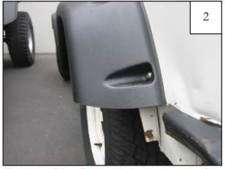
If labels have fallen off during shipping, the shorter leg of the front flare is trimmed close to the fowardmost pocket and the shorter leg of the rear flare is trimmed approximately an inch and a half from the pocket. Pictured above is the rear flare.
