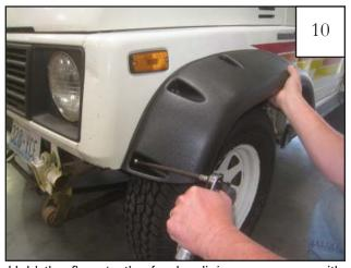
Hold the flare to the fender, lining screws up with 3/16" drilled holes and start screws into sheet metal. Once all screws are started, tighten to 2 ft•lb of torque.
