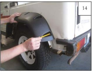
Hold rear flare in position on fender and, using a grease pencil, mark each hole location on sheet metal.
