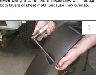
At each flare pocket, insert a Screw (SW1-0045) and run it into a Spacer (SP1-0009) until snug with the flare plastic. Use a 5/16" socket and 6" extension to prevent marring flare plastic. Wrap a layer of masking tape around Torx Bit (SW1-0052) to help it stay in the socket.
