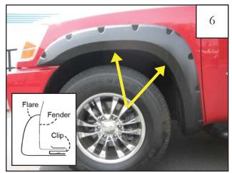
Install two Clips (CL1-0005) over fender lip, lining up the hole in clips with the holes in flare. Start Screws (SW1-0050) in each Clip. *Do not fully tighten screws*.
