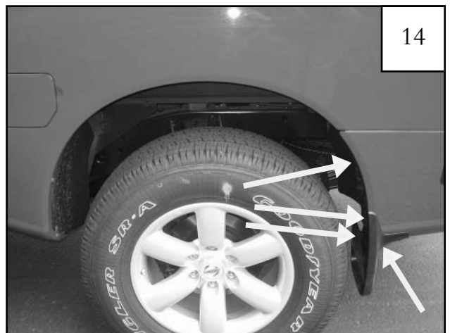
Driver Side Flare: Remove factory mud flaps if installed, and one extra unpainted screw above mud flap.
