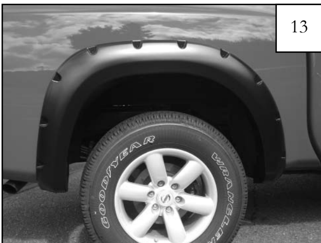
Passenger Side Flare: Completed rear flare installation.
